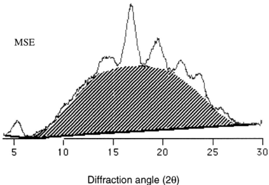
*Figure 12 – Diffraction patterns with amorphous regions fitted with an arbitrary semi-circle. Figure from (Cheetham; Tao, 1998)*
