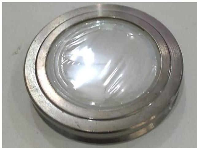
*Figure 14 – Adapted sample holder with a fake bottom made of Mylar® film. Photo taken by the author.*
