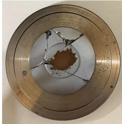
*Figure 13 – Damaged oriented silicon sample holder. Photo taken by the author.*
