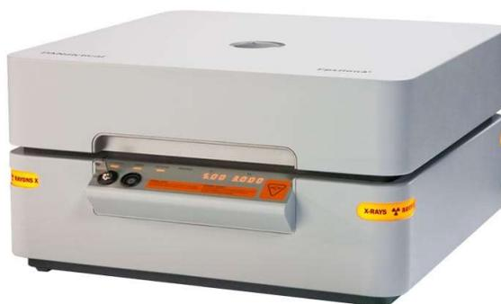
**Figura 38:** Espectrômetro PANalytical, EPSILON 3 XL.
