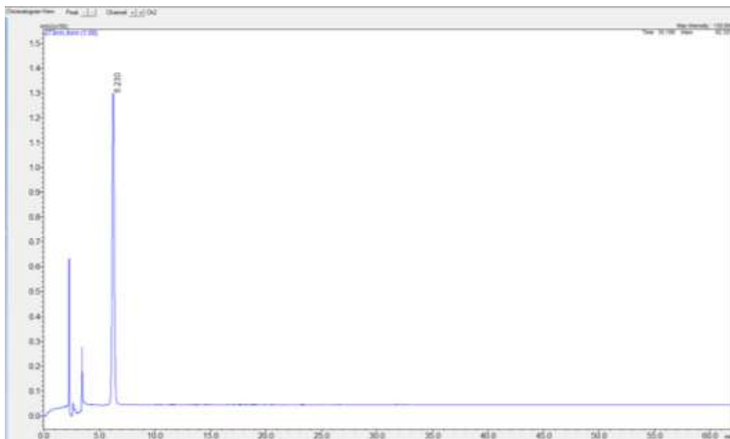
Figura 5- Teobromina a Tr 6,230 min – UV 273 nm
