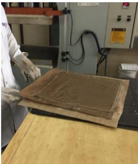
**Figura 68** - Compósito de caroço de açai
